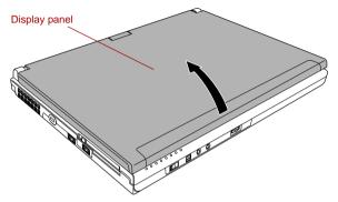
Figure 1-4 Opening the display panel
